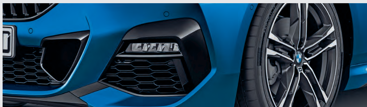
LED Fog Lights increase short-range visibility in fog or precipitation, improving night-time driving safety.
