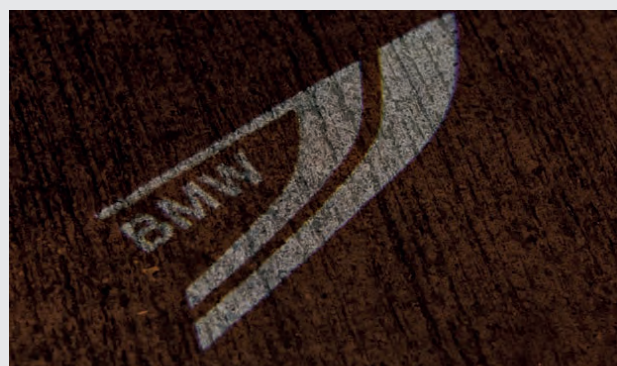
The Lights Package also includes a welcome greeting. When the vehicle is unlocked, an LED light source in the driver's-side exterior mirror projects onto the ground.
